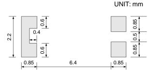
Note: Please make sure that there is no electric wire line under SSP-T6 on the circuit board.
