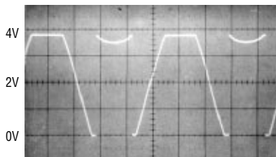
LM324, LM358, OP-20 EXHIBIT OUTPUT PHASE REVERSAL
