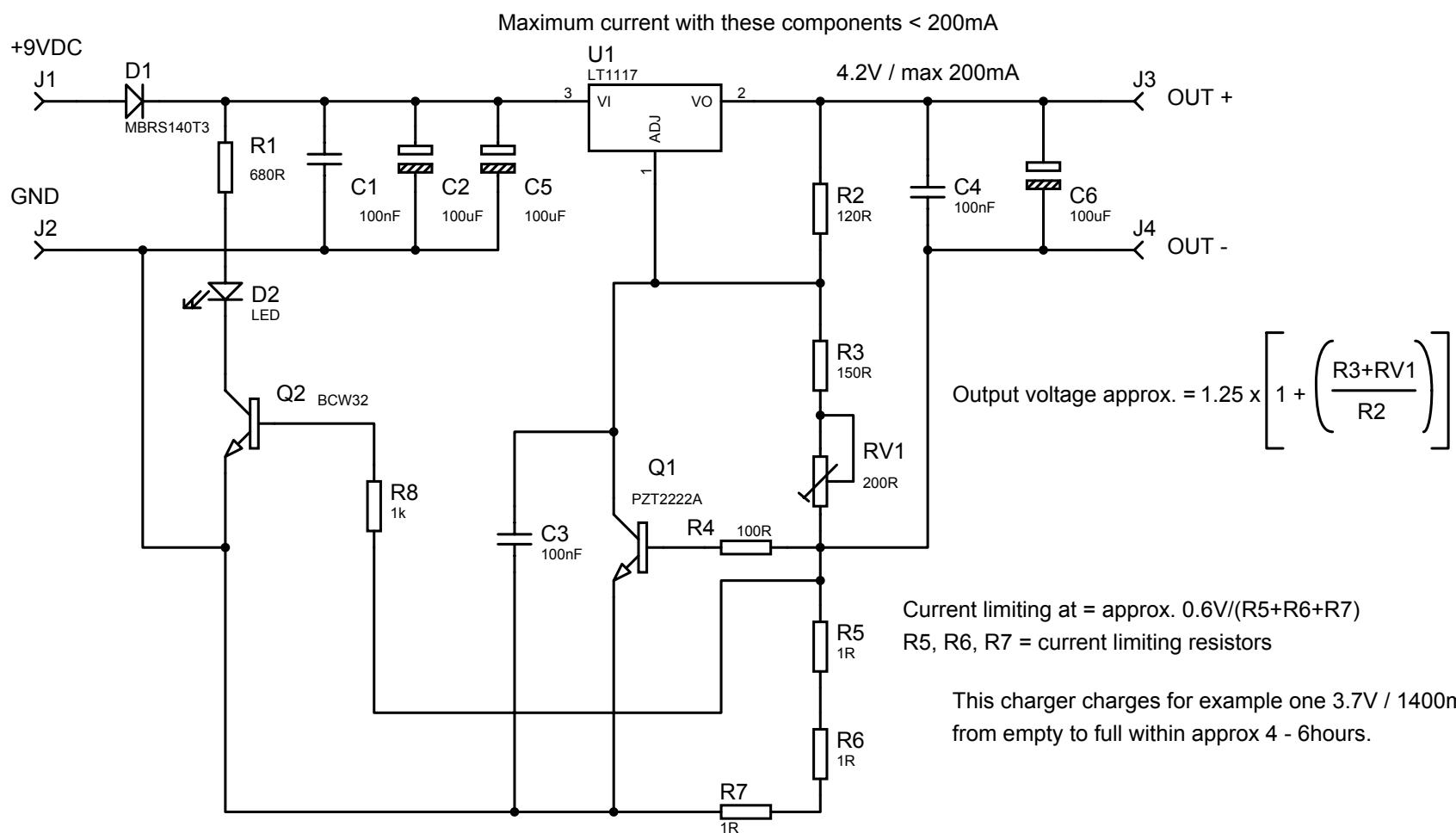
9VDC/200mA unregulated powersupply is enough to supply sufficient voltage and current.
