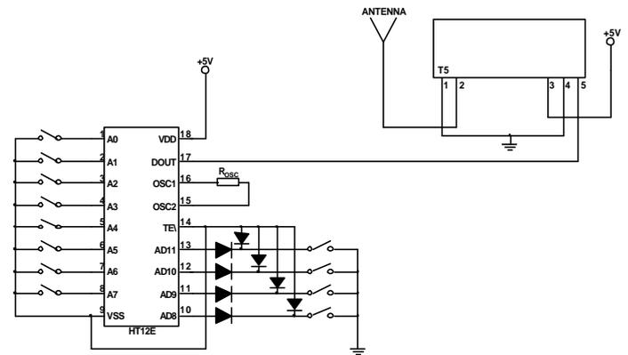
Figure 4: T5 Transmitter Application Circuit
