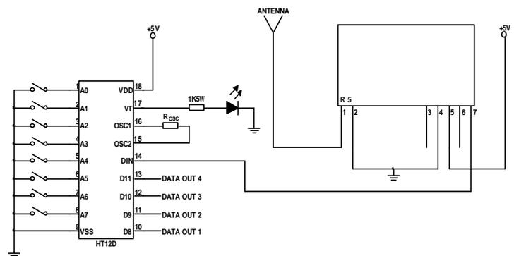
Figure 5: R5 Receiver Application Circuit
