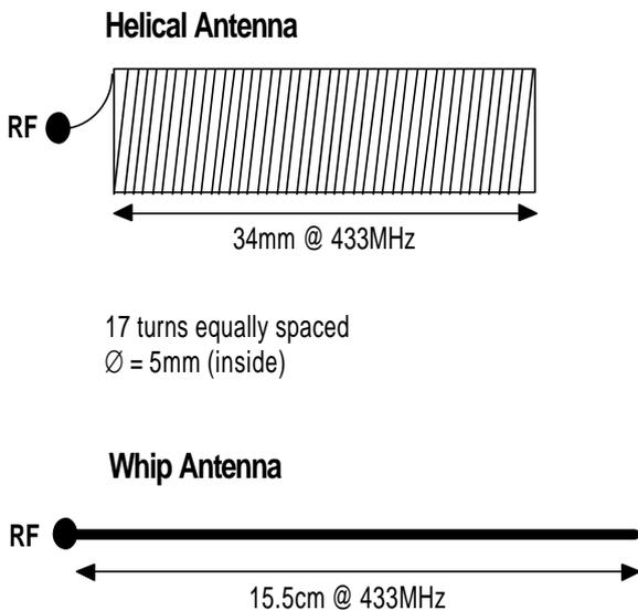
Figure 3: Antenna Configurations To Be Used With The T5 & R5 Modules
