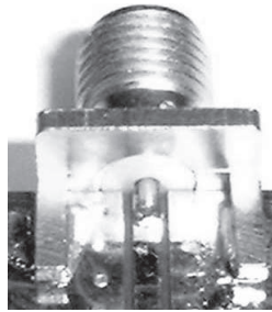
Figure 13. Soldering details of connector fingers to upper ground plane.
