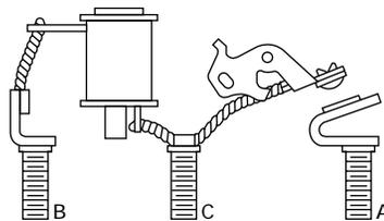
Controls two circuits from common source with high-inrush capability
