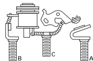
Controls two circuits from common source; provides extra (25x) high-inrush capability
