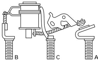
Controls two circuits, with voltage trip capability, from common voltage source
