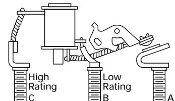
Allows multiple ampere ratings in one breaker; high-inrush capability
