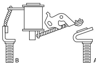
Standard circuit protection; coil in series with contacts
