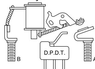
Remote indicating auxiliary switch with two separate circuits
