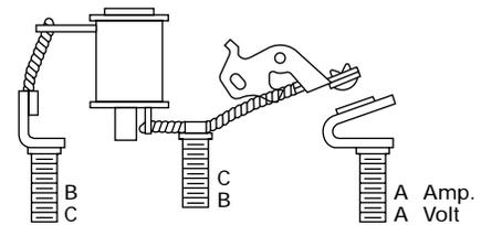
Controls two circuits from common source
