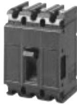
This rugged EH-frame breaker offers all the advantages of a completely magnetic, three-pole breaker with 10,000A interrupting capacity for a less costly, smaller circuit breaker. Compact, environmentally stable. To 100A at 480V AC and 250V DC.
