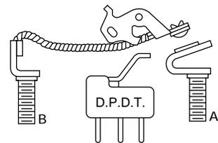
Remote indicating switch with two separate circuits
