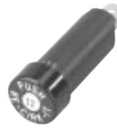
Fuse-switch provides ON/OFF control and fuse protection in a single low-cost component. Its use eliminates a hole and interconnecting wiring and makes it easy to re-fuse from the front panel. It accepts standard 1/4" diameter by 1-1/4" fuses. An adapter is available for 5 mm x 20 mm fuses. Can be supplied for NO or NC operation.
