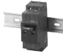
DM/S circuit breakers snap easily into a standard 35 mm DIN rail and may be mounted or detected without moving other breakers on the rail. They provide all the advantages of hydraulic-magnetic circuit protection including freedom from heat-induced nuisance tripping and a wide choice of time delay ranges. Available with auxiliary SPDT switch for alarm or control purposes.
