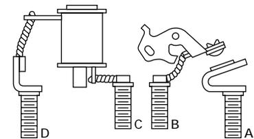
Controls two circuits from separate sources with high-inrush capability on one circuit
