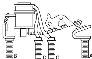
Controls two circuits, with voltage trip capability, from two separate voltage sources; high-inrush capability
