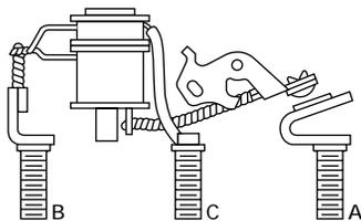
Controls two circuits, with voltage trip capability, from common voltage source; high-inrush capability
