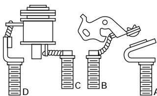
Controls two circuits from separate sources; provides extra (25x) high-inrush capability on one circuit
