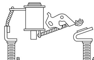
Allows circuit breaker to withstand high-inrush surges; eliminates nuisance tripping
