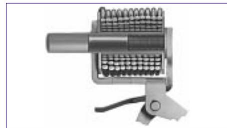
1. The HEINEMANN hydraulic-magnetic circuit breaker operates on load-current-produced magnetic flux variation in a solenoid. The coil is wound around a hermetically sealed, non-magnetic tube containing a spring-loaded, movable iron core and a silicone liquid fill. With the load current either at or below the breaker's nominal rating, the magnetic flux is of insufficient strength to move the core, and it remains at the end of the tube opposite the armature.
