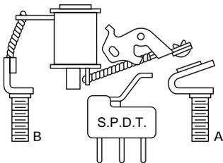
Auxiliary switch used as remote indicator to show breaker position
