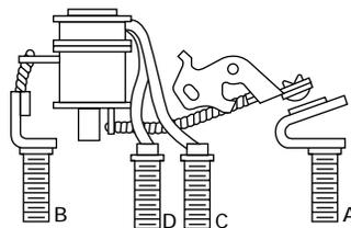
Controls two circuits, with voltage trip capability, from two separate voltage sources
