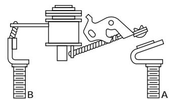
Provides extra (25x) high-inrush capability; coil in series with contacts
