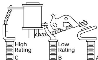
Allows two ampere ratings in one pole
