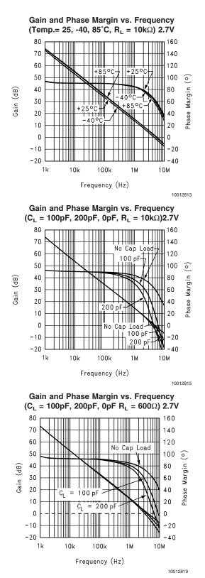
Typical Performance Characteristics Unless otherwise specified, V<sub>S</sub> = +5V, single supply,  $T_A = 25^{\circ}C.$  (Continued) Gain and Phase Margin vs. Frequency  $(C_{L} = 100 \text{pF}, 200 \text{pF}, 0 \text{pF} \text{ R}_{L} = 600 \Omega) \text{ 5V}$ 80 160 70 No Cap Load 140 60 120 100 pF CI = 50 100 0 Phase Margin 40 80 Gain (dB) C 200 pF = 30 60 20 40 10 20 0 0 = 100 pF C -10 -20 = 200 pF CL -20 -40 1k 10k 100k 1M 10M
