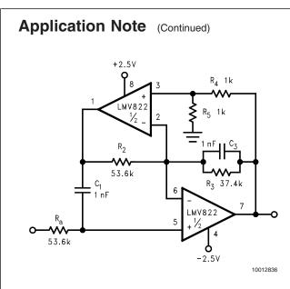
FIGURE 10. Dual Amplifier, 3 kHz Low-Pass Active Filter with a Butterworth Response and a Pass Band Gain of Times Two
