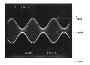
FIGURE 9. Output signal per the Circuit of Figure 8
