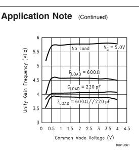
FIGURE 2. Unity-Gain Frequency vs Common Mode Voltage for Various Loads
